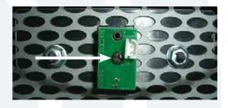
Use the phillips head screwdriver to remove one screw near the center of the led PCB assembly.
